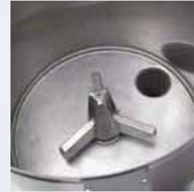
Residual water drain
